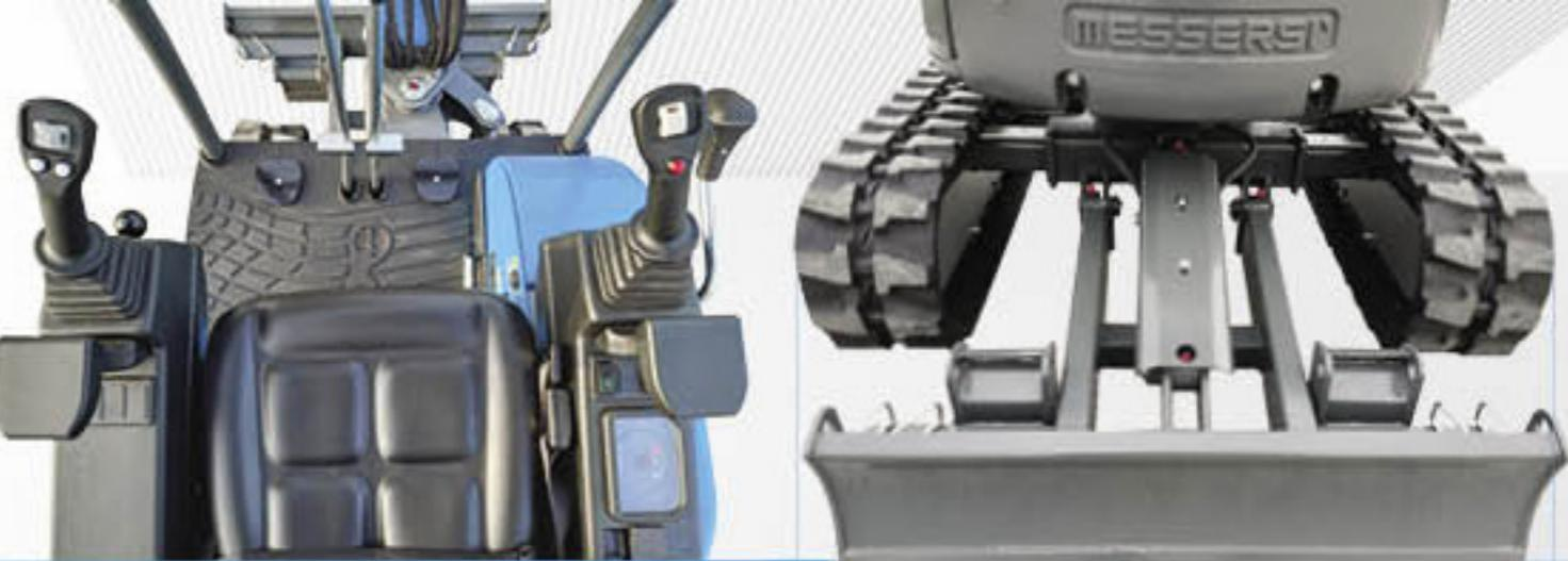
1 M16U - Joysticks with electro-servocontrols (roller).
