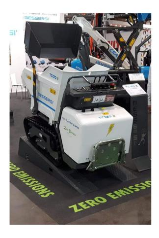
The TC120e, has now important and interesting innovations in the joysticks and inverters internal electronic management by the CAN bus system, which makes simpler all the operations, from assembling phases to general maintenance and set-up. This opens a lot of new possibilities in the problem solving via software, because the machine management parameters can be changed remotely
