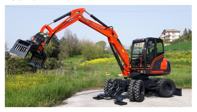
Intermat 2018 also saw the launch of the new mini-digger M18DS, with the acronym DS indicating "Double Speed" (two speeds hydraulic driving motors). Born as an evolution of the very successful M18BE, with new design and enhanced in the performance by the addition of modern electro-proportional joysticks.
