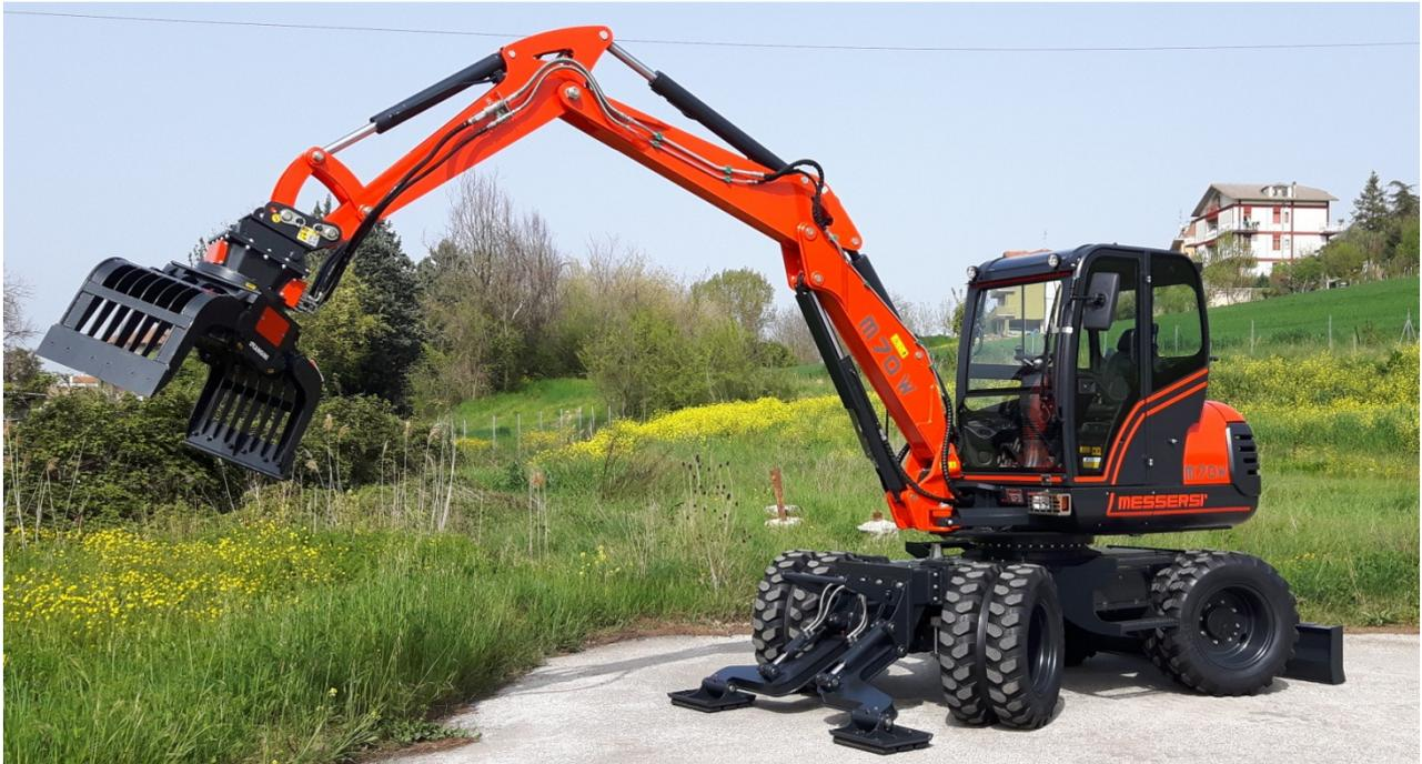
Intermat 2018 also saw the launch of the new mini-digger M18DS, with the acronym DS indicating "Double Speed" (two speeds hydraulic driving motors). Born as an evolution of the very successful M18BE, with new design and enhanced in the performance by the addition of modern electro-proportional joysticks.
